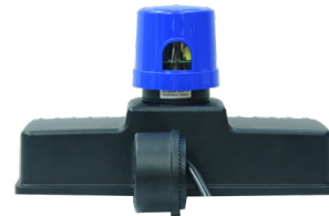
Daylight Sensor ETG-SEN-7P-MV-DIM *Turns on/off at 100 lux *Dims to 50% at midnight and brightens to 100% the last hour before sunrise
