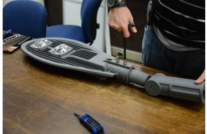
On the R200 unit, secure the arm to the unit by tightening the 8mm hex screws on the front (max 60 in-lbs).
