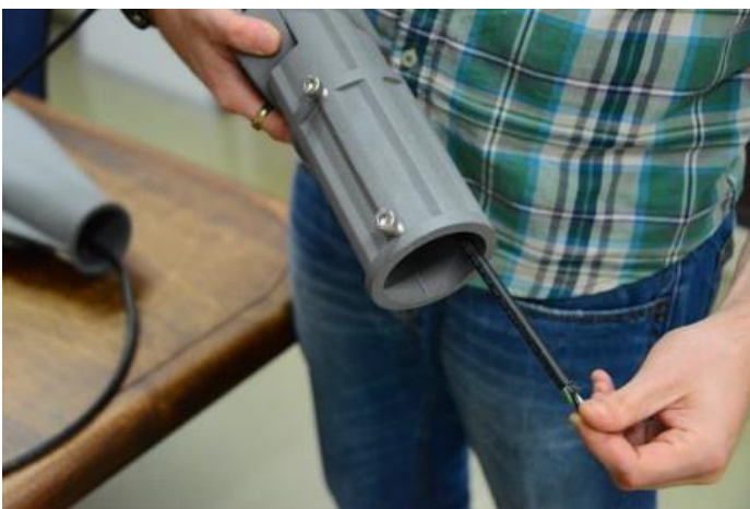
Pull the burial wire through the other end. This will be the end with the two 6mm hex adjustable screws.
