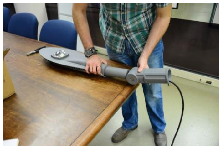
Slide the arm up and fit it into the unit. This part of the process will be the same for each unit.
