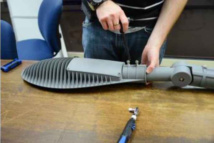
On the R80 unit, secure the arm to the unit by tightening the 6mm hex screws on the back (max 60 in-lbs).
