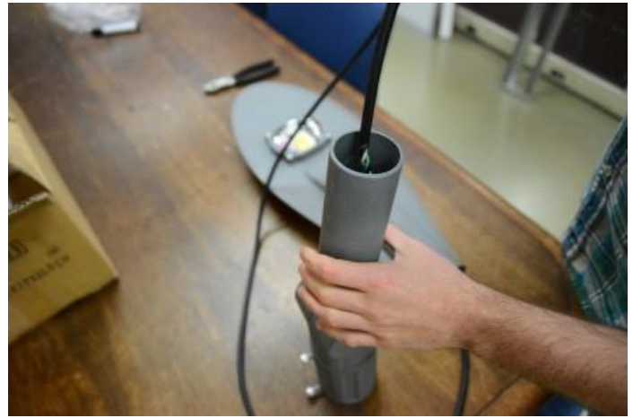
To attach the arm, run the burial wire through the arm, starting from the narrower end of the tube.
