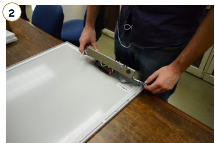
Back of Flat Panel showing wiring/power casing
