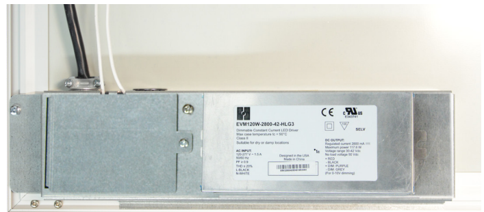
Back of Flat Panel showing wiring/power casing
