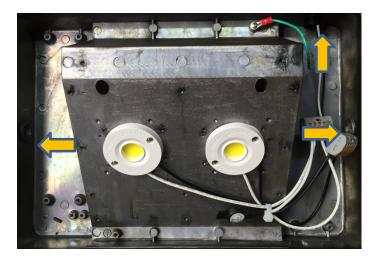
The service wire for the fixture should enter using one of the three 1/2" conduit points on the fixture. Be sure to make proper water tight conduit connections that follow your local code.
