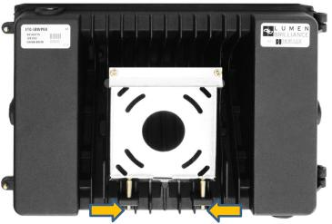
The LBWP series uses a mounting bracket to secure the fixture. There are two 3mm Allen set screws holding it in place. Remove these to start the mounting process.
