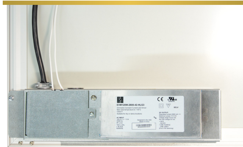
Back of Flat Panel showing wiring/power casing
